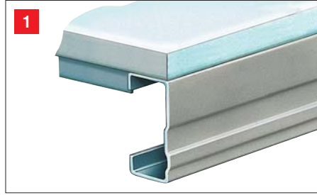
1. Medium Duty 'C' Section Beam (2LSC) - use as a support for chipboard or steel shelf panels. Beam lengths range from 1050-1800mm. Panels 300/374/600mm wide.
